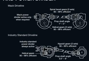
Cast ductile iron axle housings and top-mounted carriers stand up to high gross vehicle weight and provide an additional 2" of ground clearance over conventional rear axles. Near straight driveline angles provide more efficient and reliable performance.
