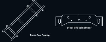
The backbone of Mack's pump chassis is our 120 ksi steel frame rails, engineered for long-term durability. A wide cross-section means heavy loads are absorbed without stressing the frame system. Formed steel plate crossmembers deliver unrivaled strength through the entire frame ladder.
