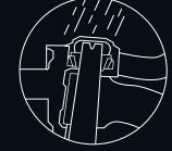
Mack FXL axles use a self-locking kingpin with an internal thrust bearing. That means no exposure to the elements and no bearing contamination. Simple. Strong.
